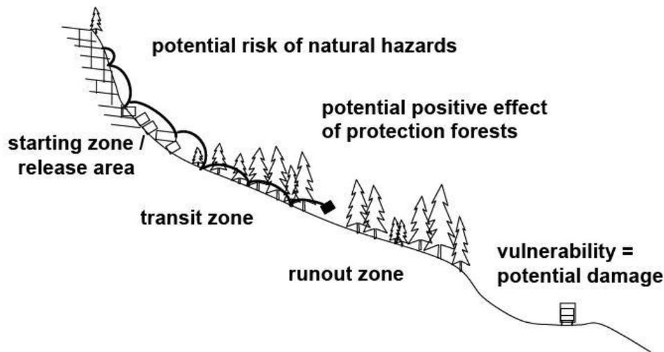
Figure 2: schematic sketch of starting, transit and runout zone of rocks
