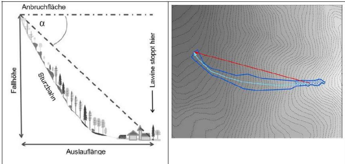
Figure 3: schematic description of the energy line approach: Fahrböschungslinie (cyan) and direction vector (red) of a documented avalanche in tyrol
