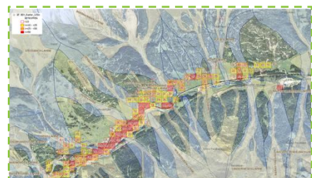
Settlement grid (125 m grid) - Stanzertal (Rosanna) / section Pettneu to St. Anton am Arlberg (Test-bed Arlberg by N. Wergles & I. Schnetzler)
